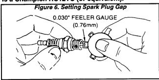
Clean the Spark Plug and reset its gap to 0.030 inch (0.76mm) every 100 hours of operation. Clean by scraping or wire brushing and washing with commercial solvent. DO NOT blast clean the spark plug.
